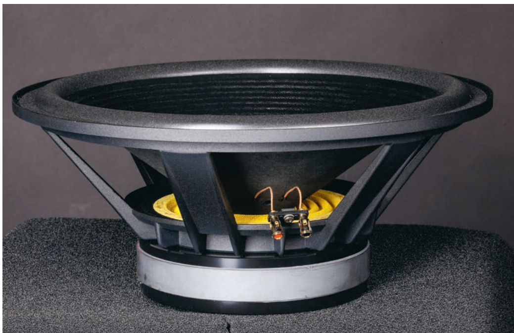
With its rigid cardboard cone and a strong die-cast basket on the one hand, but also with its foam surround and a small voicecoil, the 16-inch woofer combines PA and hi-fi genes.
